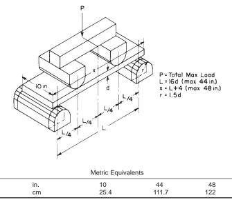
FIG. 1 Apparatus for Equivalent Uniform Load
